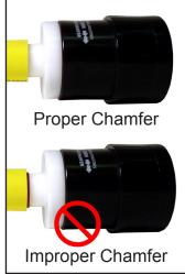
**7** Stab pipe completely into fitting entrance.
